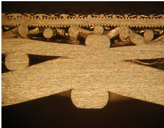
Cross Section of Poroplate® media Poroplate® is a registered trademark of Purolator-Facet
