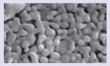
Sintered TiO<sub>2</sub> membrane (20,000x)
