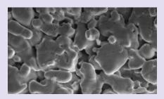
Sintered Stainless Steel membrane support (500x)
